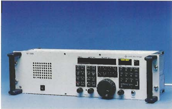
Fig. 3: Receiver Control Panel
