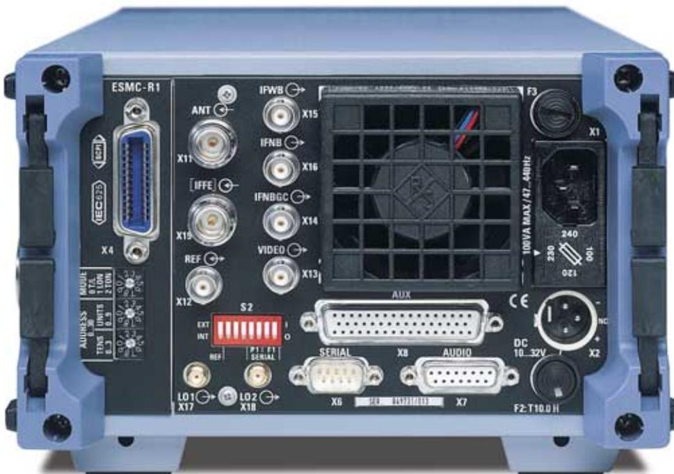
Rear of ESMC; the IEC/IEEE bus can optionally be replaced by RS232 and RS422/RS485 interface
