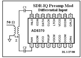
The SDR-IQ uses an AD8370 in single ended to differential conversion for its preamp as shown in the figure above left. The  $68~\Omega$  resistor in parallel with the 200 ohm input resistance of the AD8370 presents 50 ohms to
